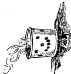
The incinerator. It is made from an old bottomless bucket with holes in it. Then it is set on a fireiron over a small fire which sets its contents burning.
